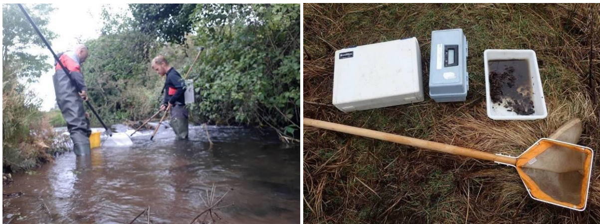
Plate 13: Electrofishing was carried out using standard gear including a battery powered electric fishing unit, dip nets and containers (left). Portable meters were used to measure certain water quality parameters and biological sampling kit required for determining macroinvertebrate community structure (right).
